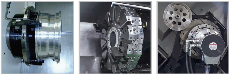
PL 500AW High speed, high precision Al Wheel turning center
